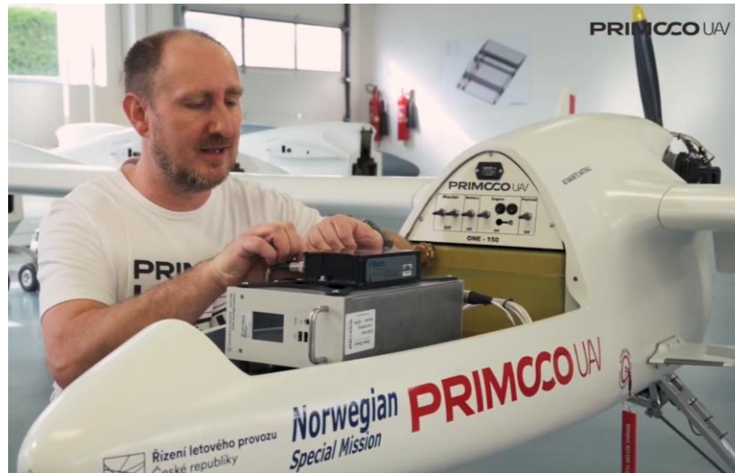
Figure 6: Primoco engineers installing the prototype UNIFIS 1000-ILS.
