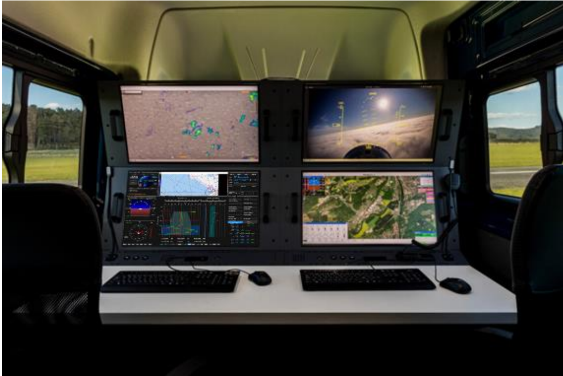
Figure 12: Integrated Ground Control Station (GCS) in the transport vehicle.
