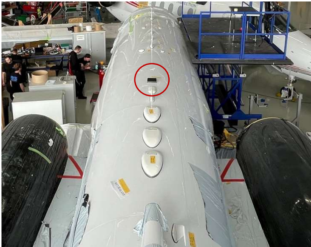
Figure 2: GNSS Anti-Jam Antenna (Marked) Installed on the Fuselage of a Flight Inspection Aircraft
