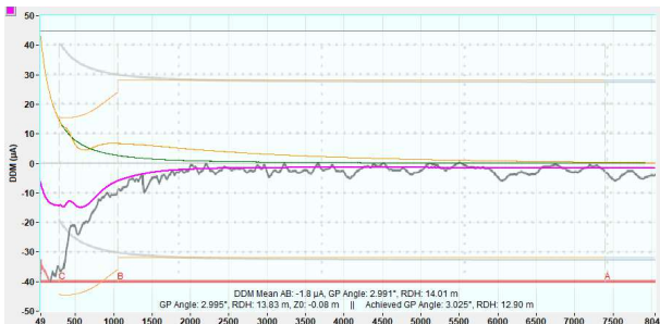
Figure 31: Simulation of incorrectly estimated aiming point (pink plot).
