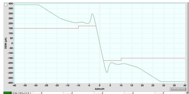
Figure 14: Simulated DDM plot with the same error
