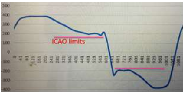
Figure 12: Ground measurement in front of localizer
