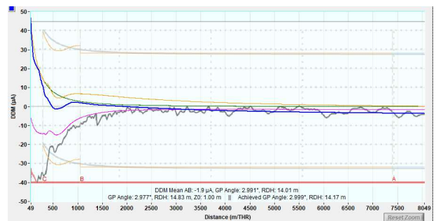
Figure 33: Simulation with rotation of the upper antenna by 4° to the runway (blue plot).
