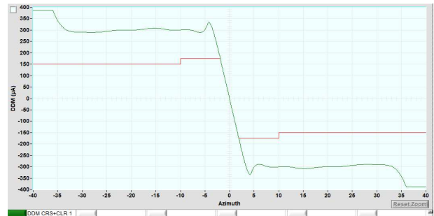
Figure 13: Expected DDM plot simulated with ATOLL.
