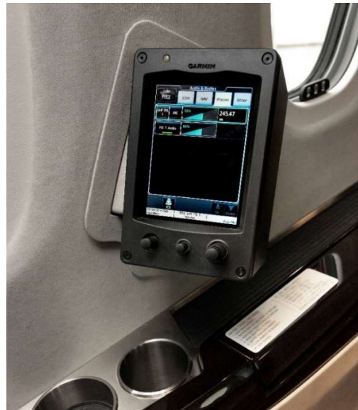
Figure 2 – Garmin GTC Controller Mounted in Aft Cabin
