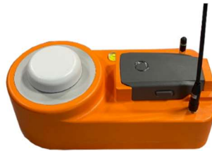
Photo 1 : Datalink RTK base station
