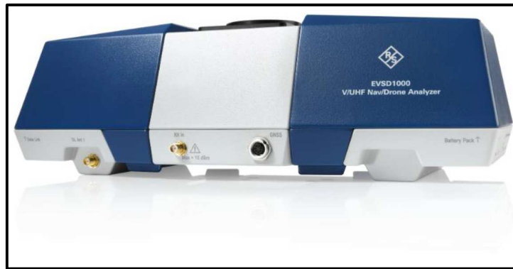
Figure 3. R&S ® EVSD1000 side view with connectors for the VHF/UHF antenna, the data link antenna, the GNSS and the two blue compartments for accessories like battery (R&S ® EVSD1-Z1) and data link module (R&S ® EVSD1-Z5)
