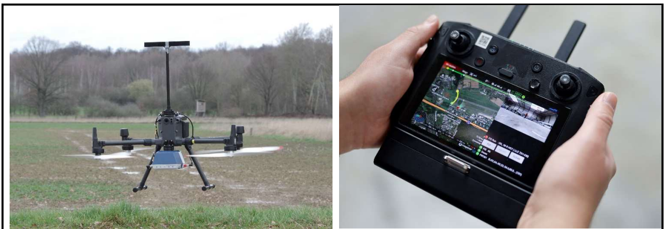
Figure 2. Left: flight of the AeroFIS® Flybot with ILS flight inspection payload R&S EVSD1000 Right: AeroFIS® Flybot Remote Control software running on the UAS remote control
