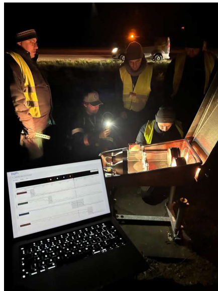
Figure 4. On-site assessment of obtained results and real-time adjustment process of PAPI Light Unit
