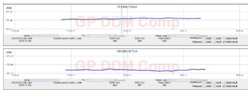
Figure 4. GP ¼ sector widths measurements during below and above offset approaches (nominally +/- 75 uA)
