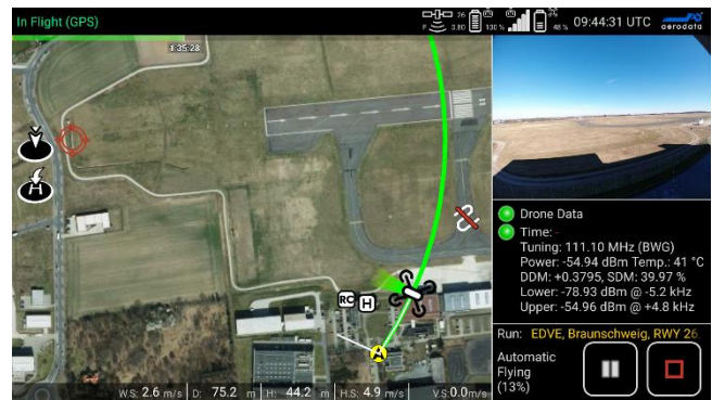
Figure 5. AeroFIS Flybot Remote Control App during ILS Localizer inspection
