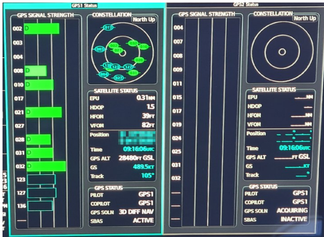
Figure 4: Example for Cockpit GPS Indication in a GNSS-denied Environment. GPS1 (Left): CRPA Anti-Jam-System. GPS2 (Right): FRPA GPS Antenna
