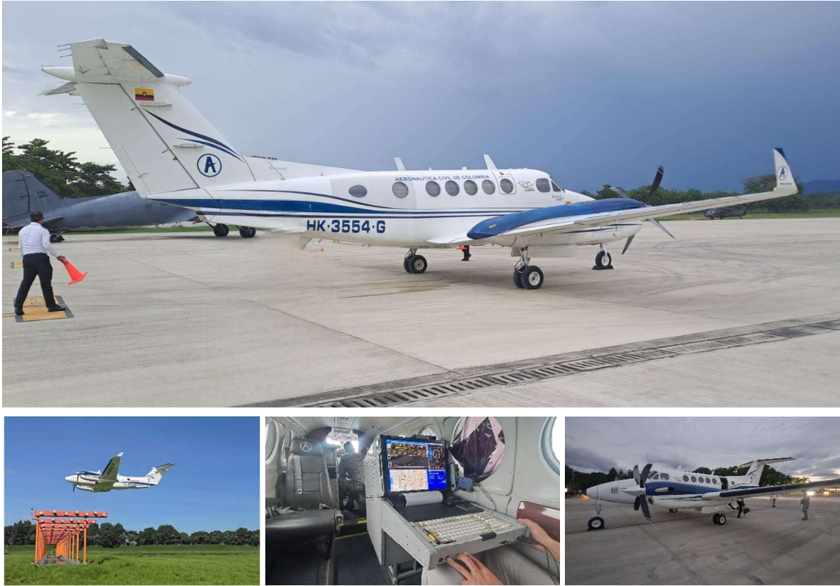
Figure 2. Beechcraft B200 Super King Air during a flight inspection procedure.
