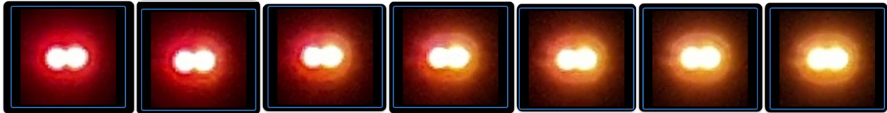
Transition representation for 2-lamp tandem halogen unit across consecutive frames in DeFI software
