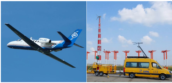
Figure 2 left: NLR Cessna Citation II flight inspection aircraft right: LVNL measurement car with localizer antenna on top, and towing an extensible mast with glide path antenna.
