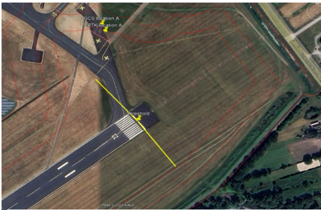
Figure 11 Arc manoeuvre ground track with ground control station and RTK reference position at Groningen airport Eelde.
