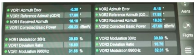
Figure 8: Screenshot Showing Nominal Deviation Ratios
