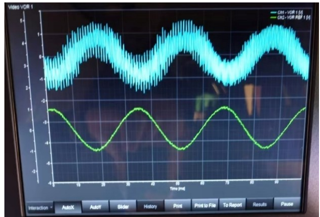
Figure 9: Oscilloscope Screenshot of the Corrected VOR Video Signal
