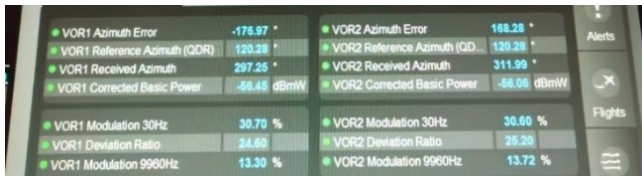
Figure 6: Screenshot Showing Excessive VOR Deviation Ratios
